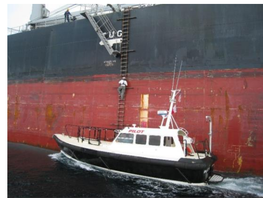
Figure MA9 - Image of a pilot boarding a vessel 246
