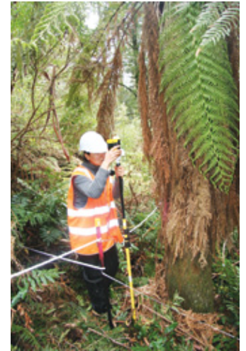
Project assistant Tapasya Arya measures the fraction of projected canopy foliage using a densitometer along star transects.
