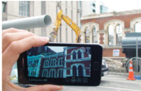
Figure 1: Person using the CityViewAR application to see virtual buildings superimposed over the real world.
