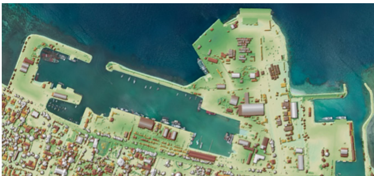
Figure 14: A digital surface model (DSM) generated by airborne LiDAR showing the port area in of Nuku'alofa, Tonga. The aerial imagery captured as part of this project is shown over the water.
