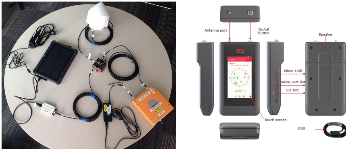
Figure 3: Original SBAS equipment configuration (left) and magicUT receiver (right).
