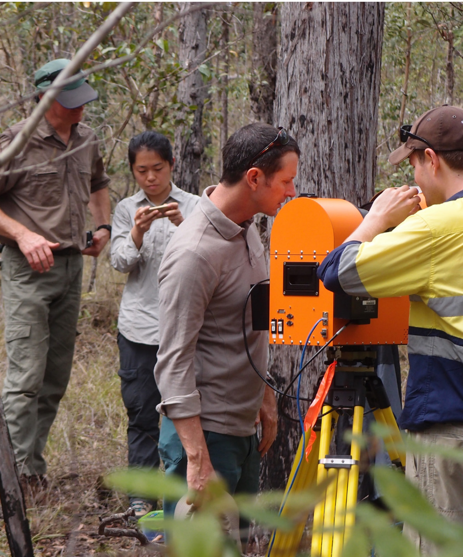
Field work using terrestrial LiDAR at Karawatha Forest, Brisbane, QLD, Australia. [Image: Mark Grant, provided by TERN.]
