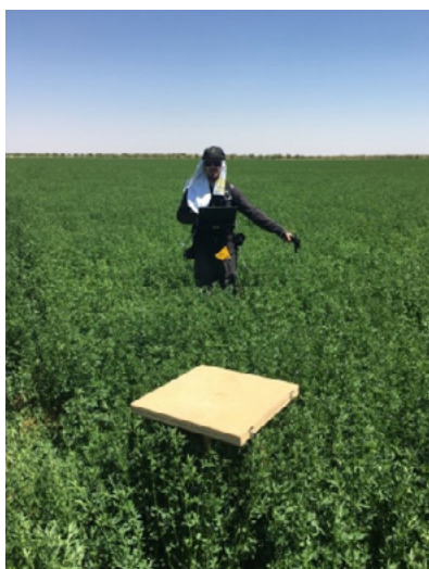
Calibration measurements of alfalfa and bare soil sites using the portable Analytical Spectral Devices (ASD) FieldSpec 4 instrument. [Image: FRM4VEG]
