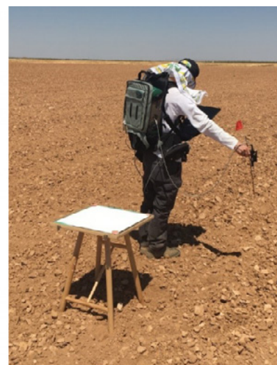
Calibration measurements of alfalfa and bare soil sites using the portable Analytical Spectral Devices (ASD) FieldSpec 4 instrument. [Image: FRM4VEG]
